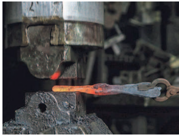
Craig Kaviar uses a World War II-era 200 pound press to flatten gun barrels. PHOTOS BY MATT STONE/COURIER JOURNAL
