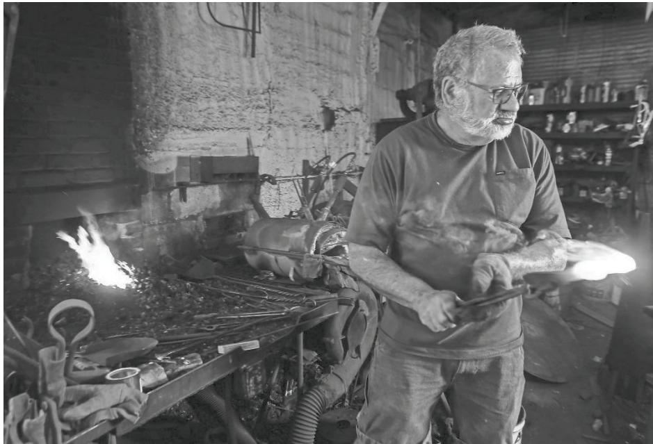
Craig Kaviar takes glowing metal that used to be a gun barrel to his anvil to hammer it into shape. He is a Louisville metal forger who takes discarded guns and transforms them into garden tools and works of art.
